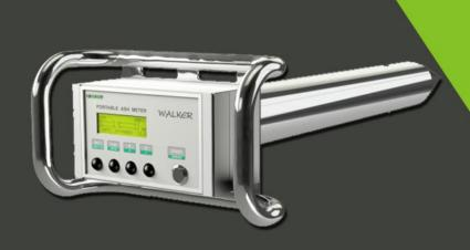
Fast, fully automated measurement of ash content in coal at storage yards, in tanks on wagons and trucks
